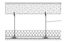
Finish Flooring Sound Mat Assembly Type Drywall Main Beam Cross Tee Insulation Gypsum Panel 2 mm Urban Surfaces 2101 Pearl (Adhered to Sound Mat) 1.3 mm Urban Surfaces FloorSilencer Pro (Adhered to Assembly) 152 mm 5000 PSI Concrete Slab 43 mm Armstrong HD8906 37.3 mm Armstrong XL8945P 88.9 mm Johns Manville Unfaced R-13 Fiberglass 15.9 mm National Gypsum Gold Bond® Fire-Shield® Type X
