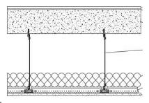
Finish Flooring Sound Mat Assembly Type Drywall Main Beam Cross Tee Insulation Gypsum Panel 2 mm Urban Surfaces 2101 Pearl (Adhered to Sound Mat)
