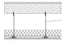
**Finish Flooring** Sound Mat Assembly Type Drywall Main Beam Cross Tee Insulation **Gypsum Panel**
