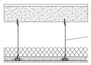
Finish Flooring Assembly Type Drywall Main Beam Cross Tee Fiberglass Insulation Gypsum Panel 5 mm Urban Surfaces Studio 12 SPC Flooring 152.4 mm 5000 PSI Concrete Slab 43 mm Armstrong HD8906 37.3 mm Armstrong XL8945P 88.9 mm Johns Manville Unfaced R-13
