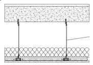
Finish Flooring Assembly Type Drywall Main Beam Cross Tee Fiberglass Insulation Gypsum Panel 6 mm Urban Surfaces SoundTec SPC Flooring 152.4 mm 5000 PSI Concrete Slab 43 mm Armstrong HD8906 37.3 mm Armstrong XL8945P 88.9 mm Johns Manville Unfaced R-13
