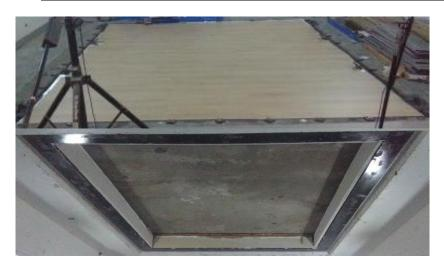
Photo 1: View of Source Chamber, Urban Surfaces SoundTec SPC finish flooring installation observed
