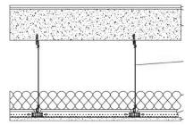
Finish Flooring Sound Mat Assembly Type Drywall Main Beam Cross Tee Insulation Gypsum Panel 3 mm Urban Surfaces 7501 Pearl (Adhered to Sound Mat) 1.3 mm Urban Surfaces FloorSilencer Pro (Adhered to Assembly) 152 mm 5000 PSI Concrete Slab 43 mm Armstrong HD8906 37.3 mm Armstrong XL8945P 88.9 mm Johns Manville Unfaced R-13 Fiberglass 15.9 mm National Gypsum Gold Bond<sup>®</sup> Fire-Shield<sup>®</sup> Type X
