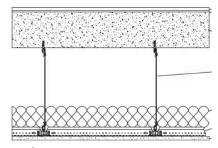
Finish Flooring Sound Mat Assembly Type Drywall Main Beam Cross Tee Insulation Gypsum Panel 3 mm Urban Surfaces 7501 Pearl (Adhered to Sound Mat)
