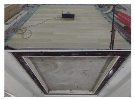
Photo 1: View of Source Chamber, finish flooring installation observed
