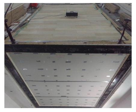
Photo 1: View of Source Chamber, finish flooring installation observed
