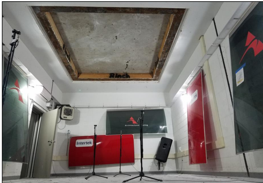
Receive Room View of Test Specimen Installation
